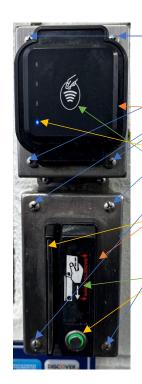
Check screws for damage or removal.
